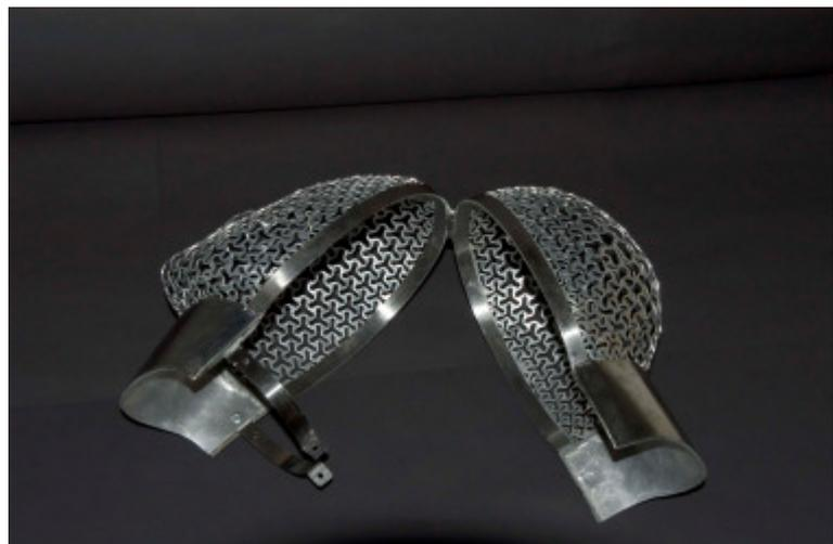
The final fitting was made using the plastic mallet while the model was wearing the head cage – very gently of course. In the end the head cage fitted perfectly. The last step was polishing the metal to get a glossy finish, which was unexpectedly – because of the many holes – a very time-consuming work.
